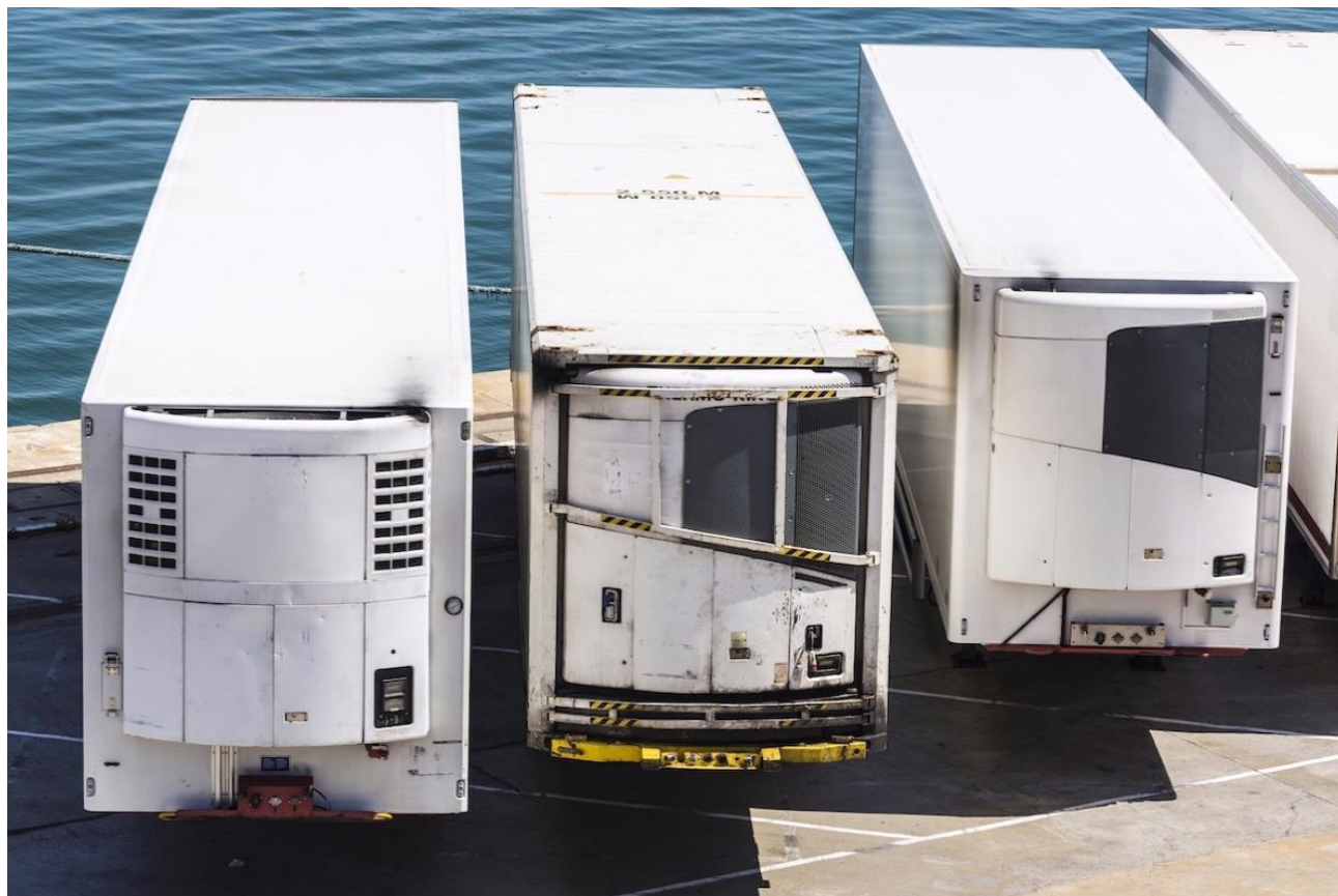
Refrigerated or reefer containers provide temperature controlled environments during transportation
