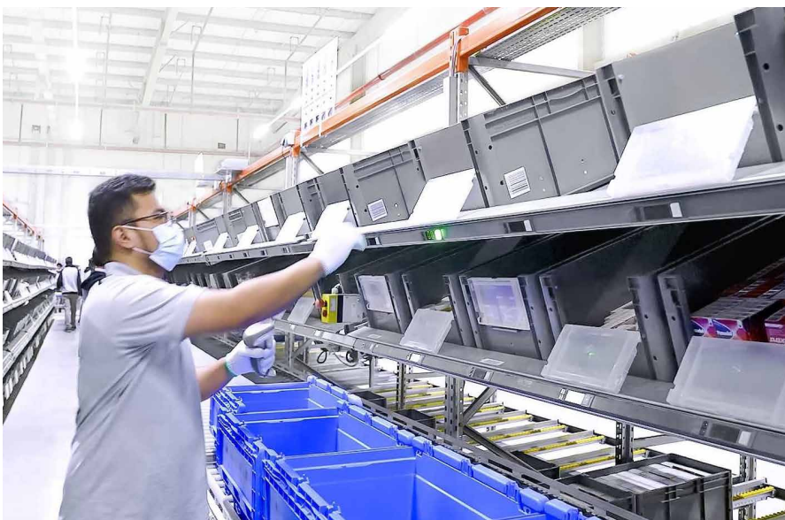
The worker in-charge is attending to one of the 64 Pick by Light workstations.
